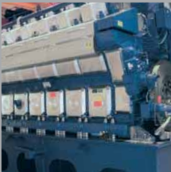
Skid mounted diesel engine
